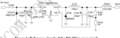
Figure 6: Reference circuit of the DC-DC power supply
