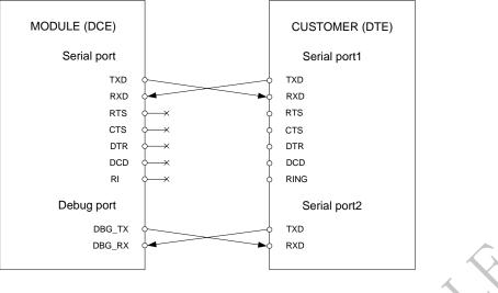
Figure 19: Connection of RXD and TXD only
