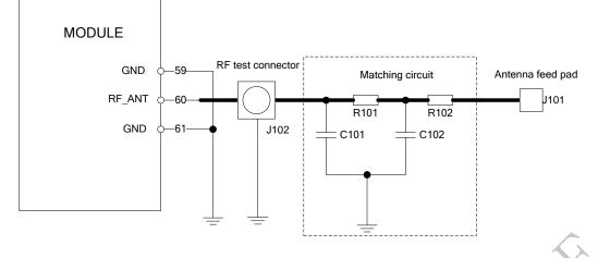
Figure 37: Antenna matching circuit
