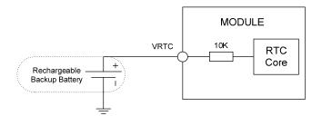
Figure 16: RTC supply from rechargeable battery
