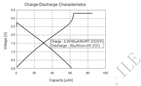
Figure 17: Seiko XH414H-IV01E Charge-Discharge Characteristic
