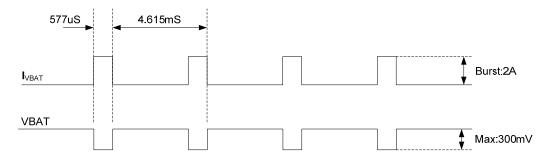
Figure 7: VBAT voltage drop during transmit burst
