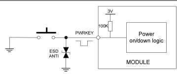
Figure 10: Powered on/down module using button
