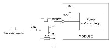
Figure 9: Powered on/down module using transistor
