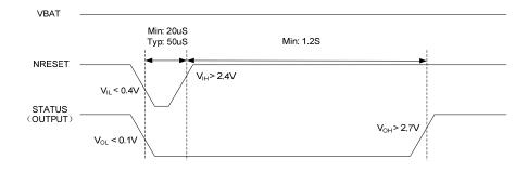
Figure 35: Reset timing
