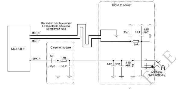
Figure 24: Earphone reference circuit
