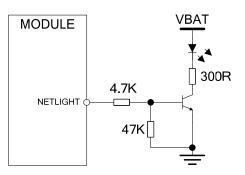
Figure 34: Reference circuit of NETLIGHT
